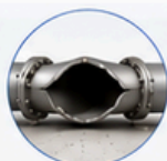
VACUUM CONDITIONS AND PIPE COLLAPSE
